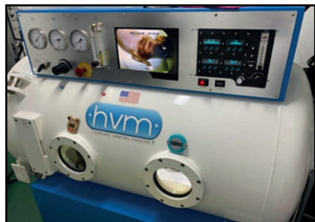
Figure 2. Hyperbaric chamber* used in the treatment of a necrotic wound caused by snakebite ( Bothrops jararaca ) in an 8-year-old dog. *[Model HVM-M1 ® - length = 1.37 m, external diameter = 83 cm, height = 1.5 m, weight = 300 kg, pressure up to 3 ATM].
